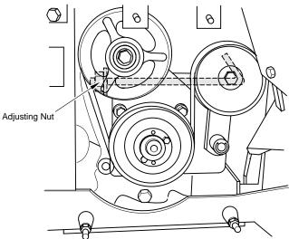
Figure 6-9 Engine Belt Adjustment
